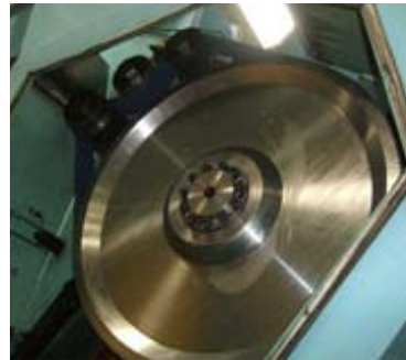
A synchronous belt drive fit into the same limited space, needs no lubrication, and has a two year lifespan
