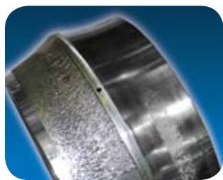
Even with such severe damage, SKF was able to remanufacture the bearing using its vast knowledge and expertise.
